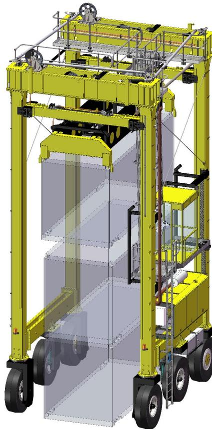
**easy bi-directional operation** - the side mounted cab and 4 wheel steering means that the machine handles the same in either direction - increasing driver efficiency.
