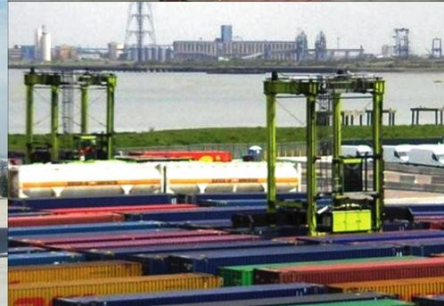
A dependable high capacity straddle carrier designed for intermodal terminals, trucking terminals, small ports and logistics centres. Comes in 1-high, 2-high and 3-high models.
