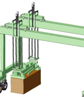
**gantry types** - choice of single beam, double beam, dry land, over water or on-barge.
